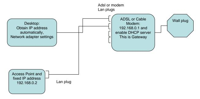
For security reason it is good idea configure the first router as bridge and connect access point and the second router to it. The second router can be NAT mode and give secure SOHO network.
